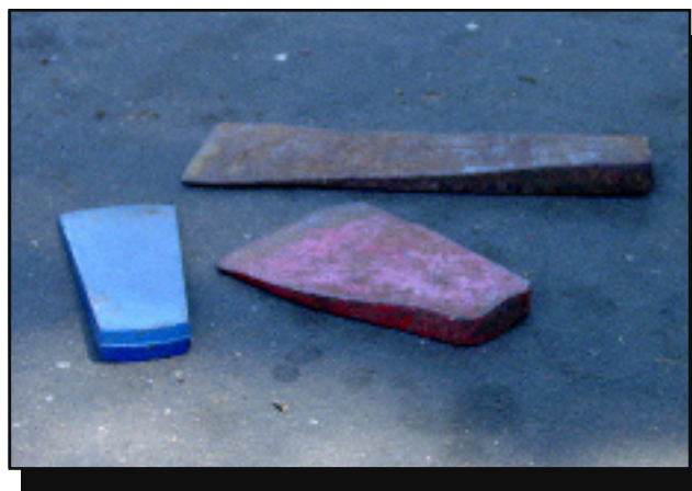
Figure 39—Traditional metal wedges used for bucking and felling.
