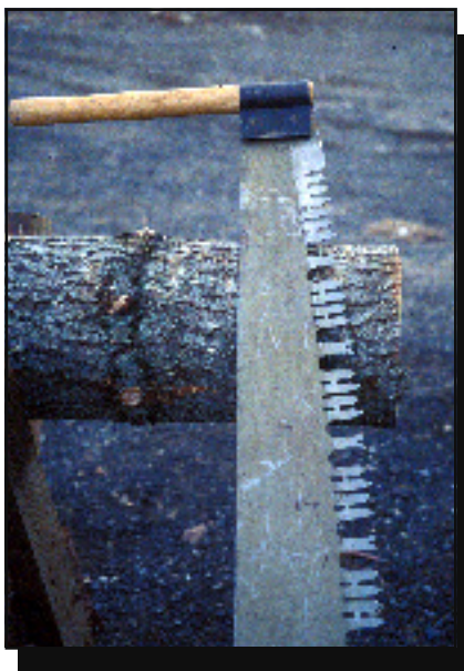
Figure 12—This vintage, but unused, Peugeot saw has its handles permanently fastened with rivets. The saw still has its original protective coating.
