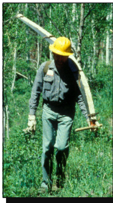
Figure 34—Transporting a crosscut saw to a jobsite by carrying the saw on the shoulder with the teeth facing outward. Saws need to be sheathed when they are carried for long distances.
