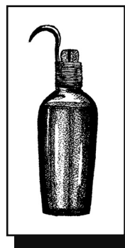
Figure 44—A traditional oil bottle applies liberal amounts of saw lubricant. The hook held the bottle to the log, conveniently within reach.— Now You're Logging , by Bus Griffiths, with permission of Harbour Publishing, Madeira Park, BC, Canada
